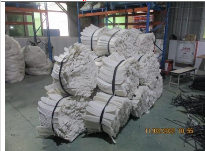
The semi-finished products in the peeling station were put on the ground directly
