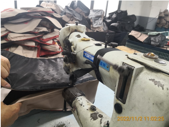
Eye protector baffle were not equipped on the 20% of the sewing machine
